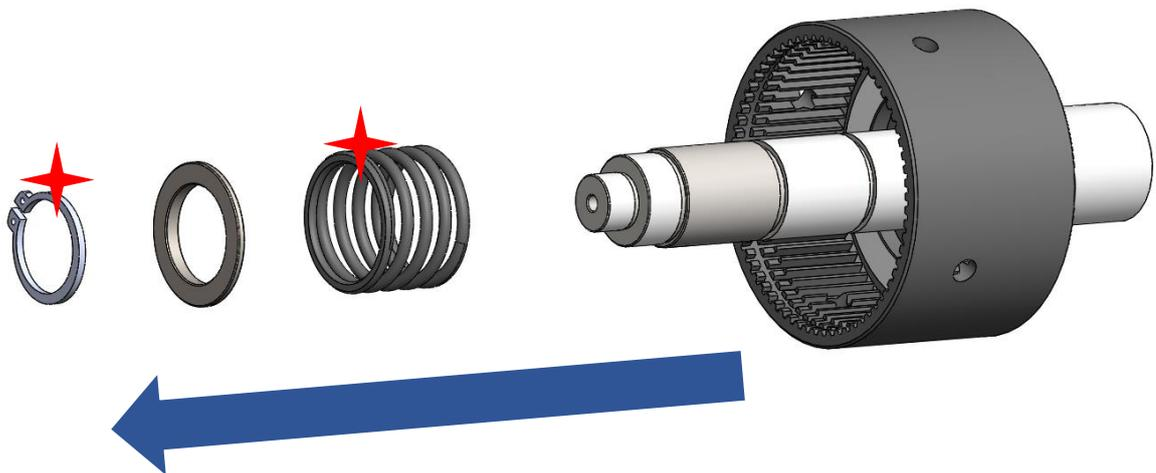
11. Snap ring on the clutch shaft could be removed to disconnect the clutch case and clutch shaft.
