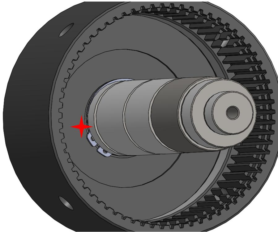
12. Change the o-ring after separating the clutch case, piston and clutch shaft.
