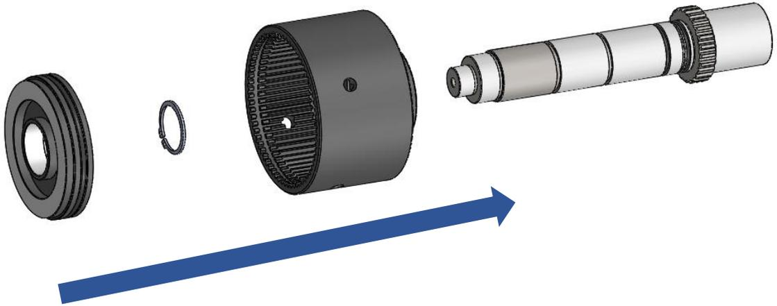
14. Spring, washer and snap ring should be assembled in a row.
