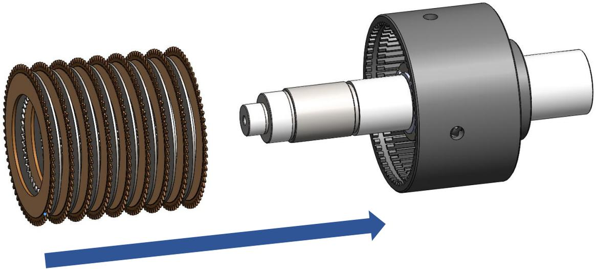
16. Insert part and snap ring should be assembled in a row.
