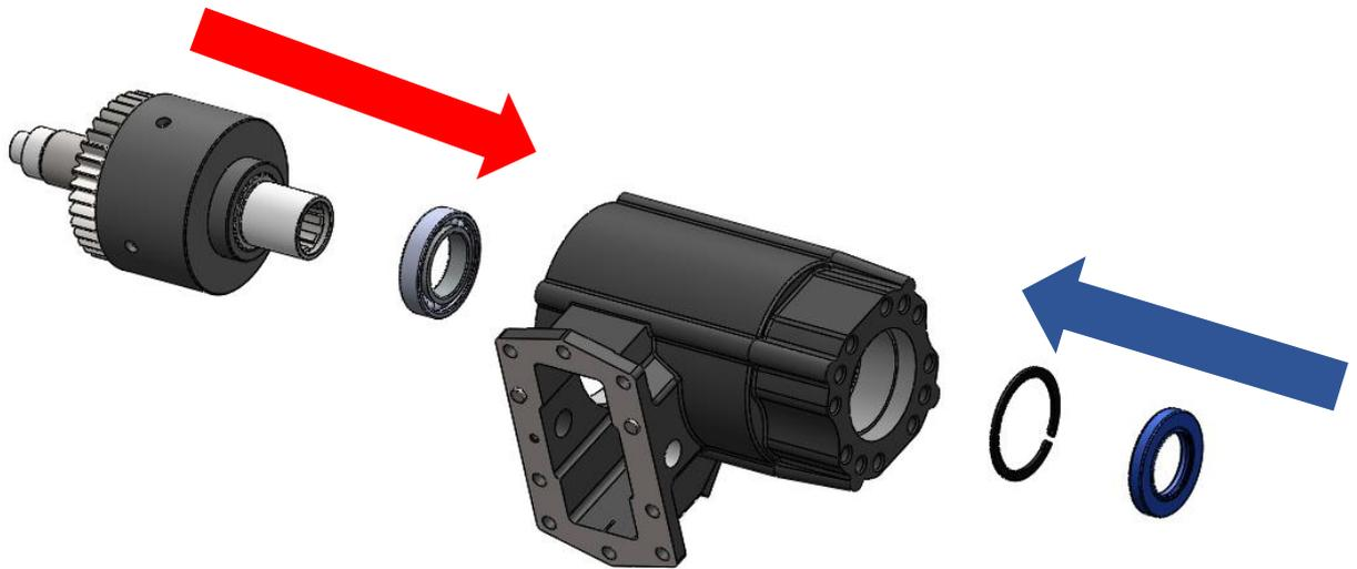
20. O-ring on the PTO cover should be greased before bearing is placed inside on the cover. Next, PTO cover should be assembled on the PTO body with 4 bolts.
