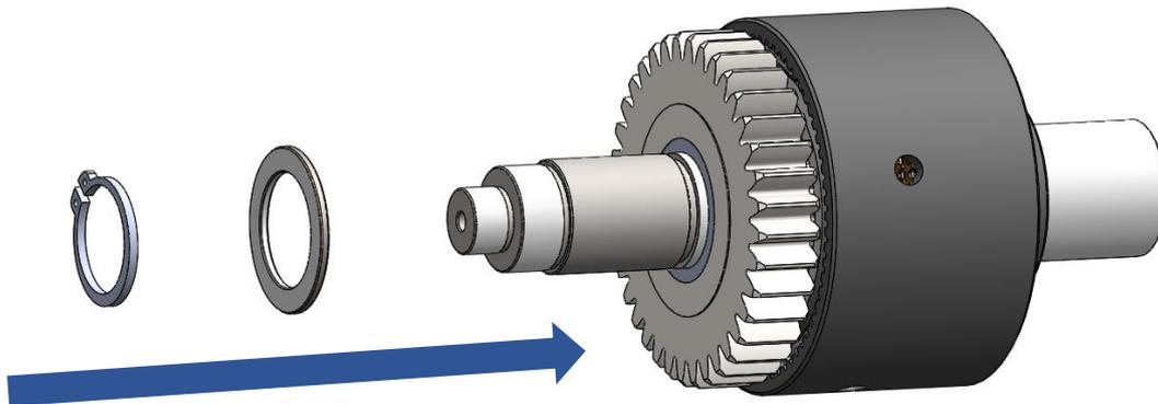
Clutch pack shall be assembled following the steps above. Air system of clutch should be checked by air inlet on the clutch shaft before mounting clutch pack to the PTO.
