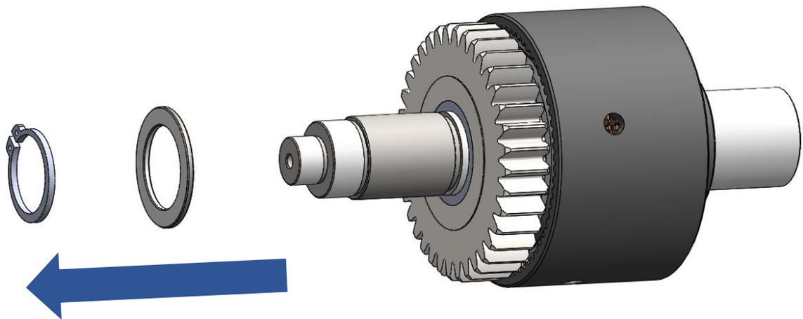
7. Clutch gear, needle bearing and washer should be removed from the clutch shaft.
