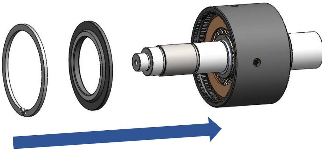
17. Gear, insert and needle bearing should be assembled on clutch shaft. Clutch gear should be matched with steel disc gears in the clutch case. Clutch gear should rotate by circular movement to match all disc gears. After that, snap ring should be assembled to fasten clutch gear and shaft.
