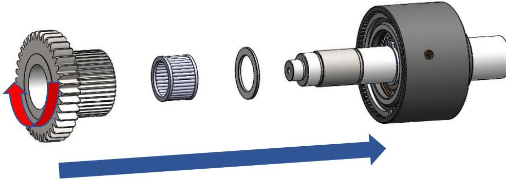
18. Washer and snap ring should be assembled after clutch gear is assembled.
