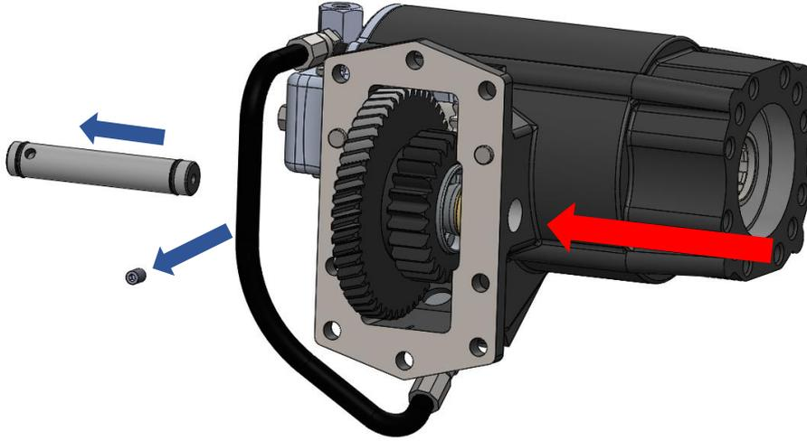
2. Main gear should be removed and be careful not to drop washers into PTO body.
