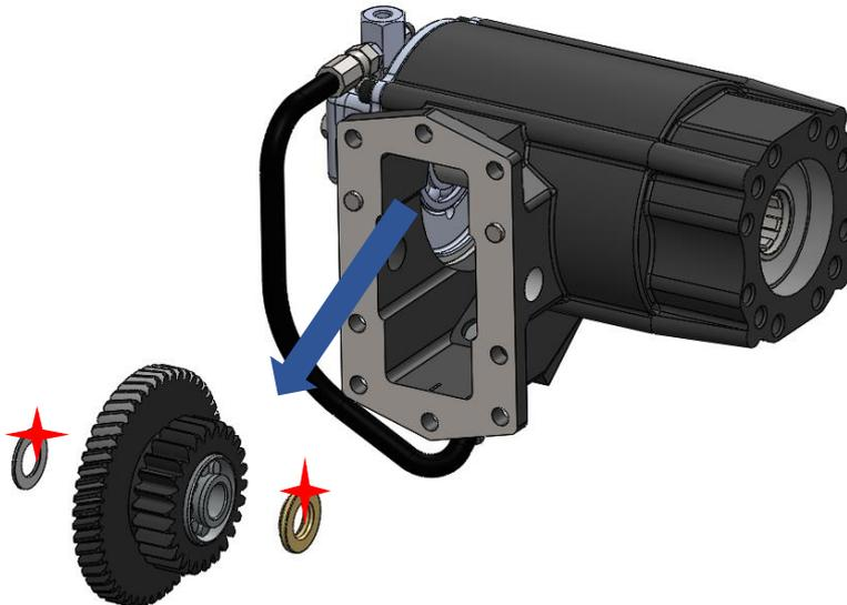
3. Hydraulic oil hose should be removed.
