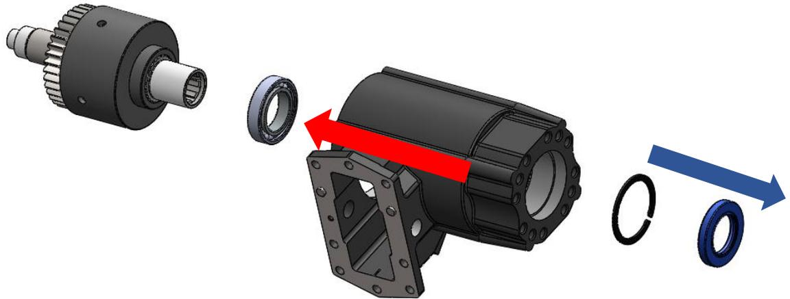
6. Snap ring and washer should be removed from the clutch shaft.
