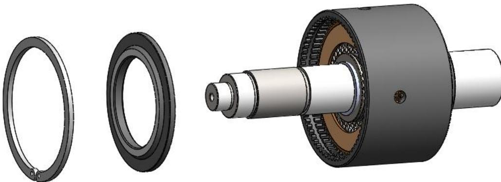
9. 9 pcs bronze and 8 pcs steel clutch discs should be removed from clutch case.
