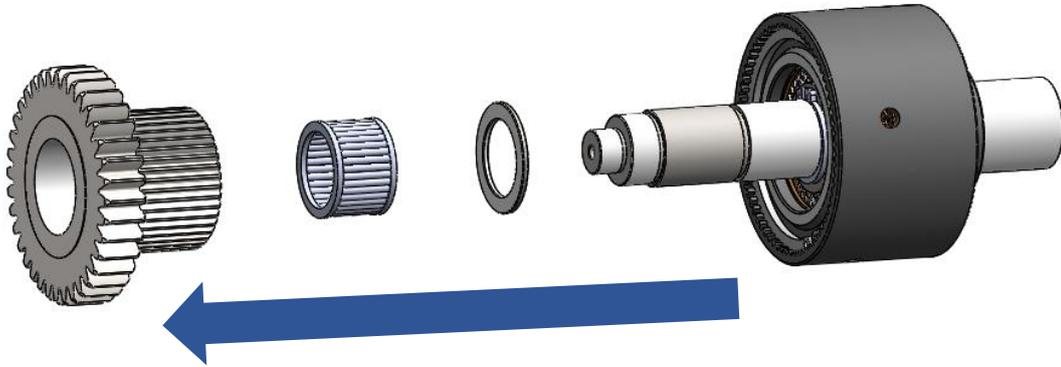
8. Snap ring and insert part should be removed from clutch case.
