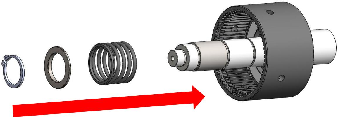
15. Clutch discs should be assembled in a row, starting with bronze disc and ending with bronze disc.
