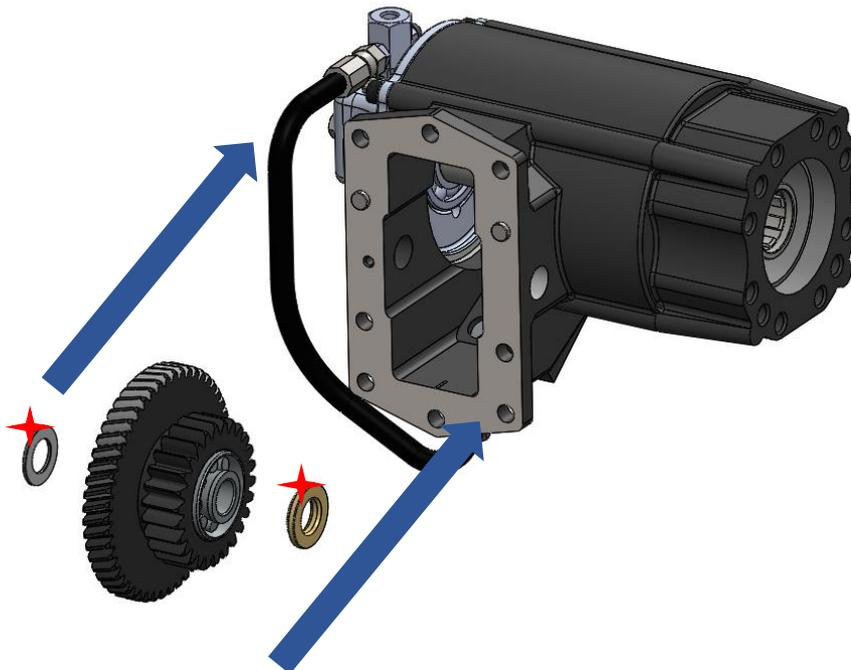
23. Shaft o-rings should be greased before reassembling the main gear shaft. Reassemble the gear shaft without orings not to cause damage to the o-rings. Put o-rings on the shaft by pushing to side and other side the shaft then fasten the stay bolt on the PTO surface.
