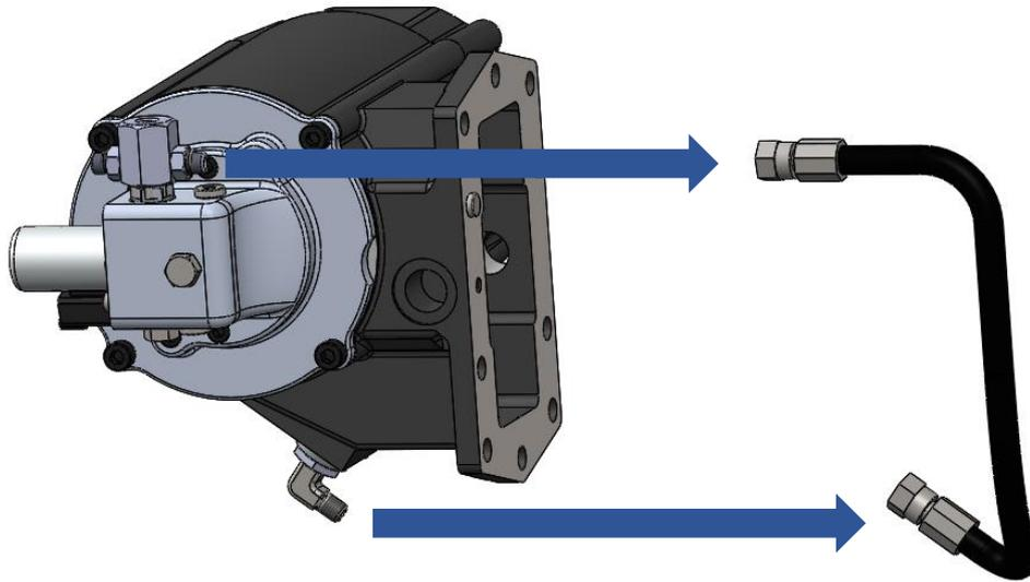
4. 4 Bolts on PTO valve side should be removed to disassemble the valve cover. Bearing on the shaft should be also removed. (Be careful if bearing stuck on the shaft)
